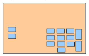
**Example 2** – this shows a monitor with two Touch Frames and 14 Touch Keys. The space within the Touch Frames not defined by a Touch Key are inactive (do not respond to touch). All areas outside a Touch Frame operate in Mouse mode. This example shows two Mouse mode "keys". e.g. Windows "Button", HTML "BUTTON" or a custom control. Other touches in Mouse mode are normally dealt with by the application event engine. However, this can be restricted – see example 3.
