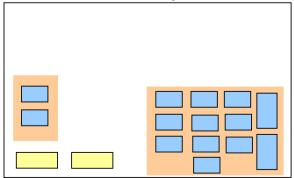
**Example 3** – this screen uses Mouse and XFS Data modes – Mouse mode is used only in a restricted area. The touch keyboard definition has 3 frames. Frame 1 has no Touch Keys. Frame 2 has 2 Touch Keys; Frame 3 has 12 Touch Keys.
