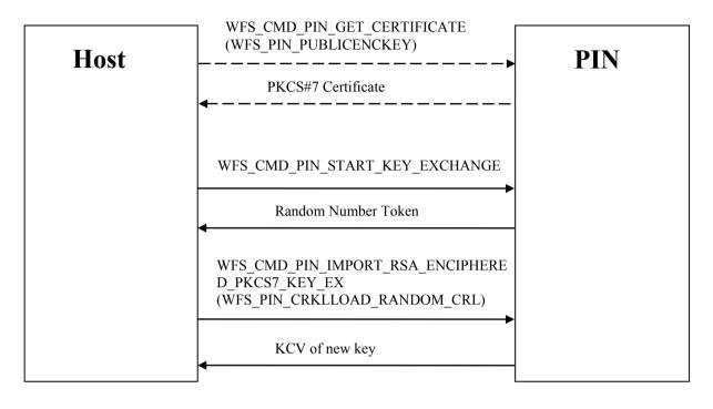
NB: Dotted lines represent commands that are only required if the PIN device encryption certificate has not been previously stored by the host.
